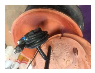
Hold the pump cord into the slot at the rear, and set the top onto the base.
