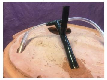
Use the 1/2" straight connector that comes with the pump. Insert the long end of the connector into the black tube the short side of
